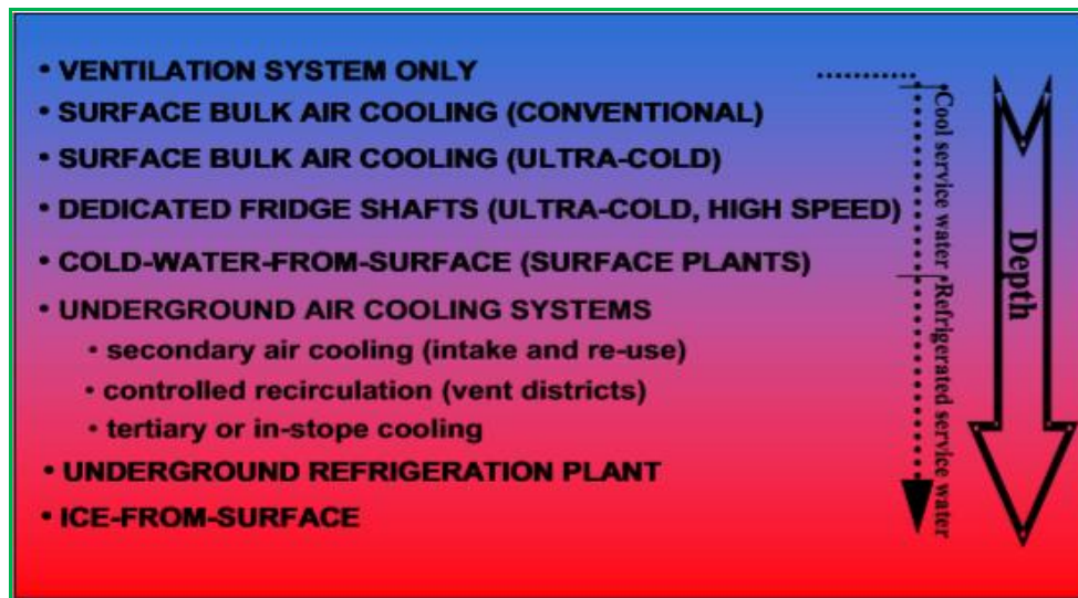
Figure 14 Generic selection of optimum cooling system as a function of depth (Mackay M. K., 2012)
