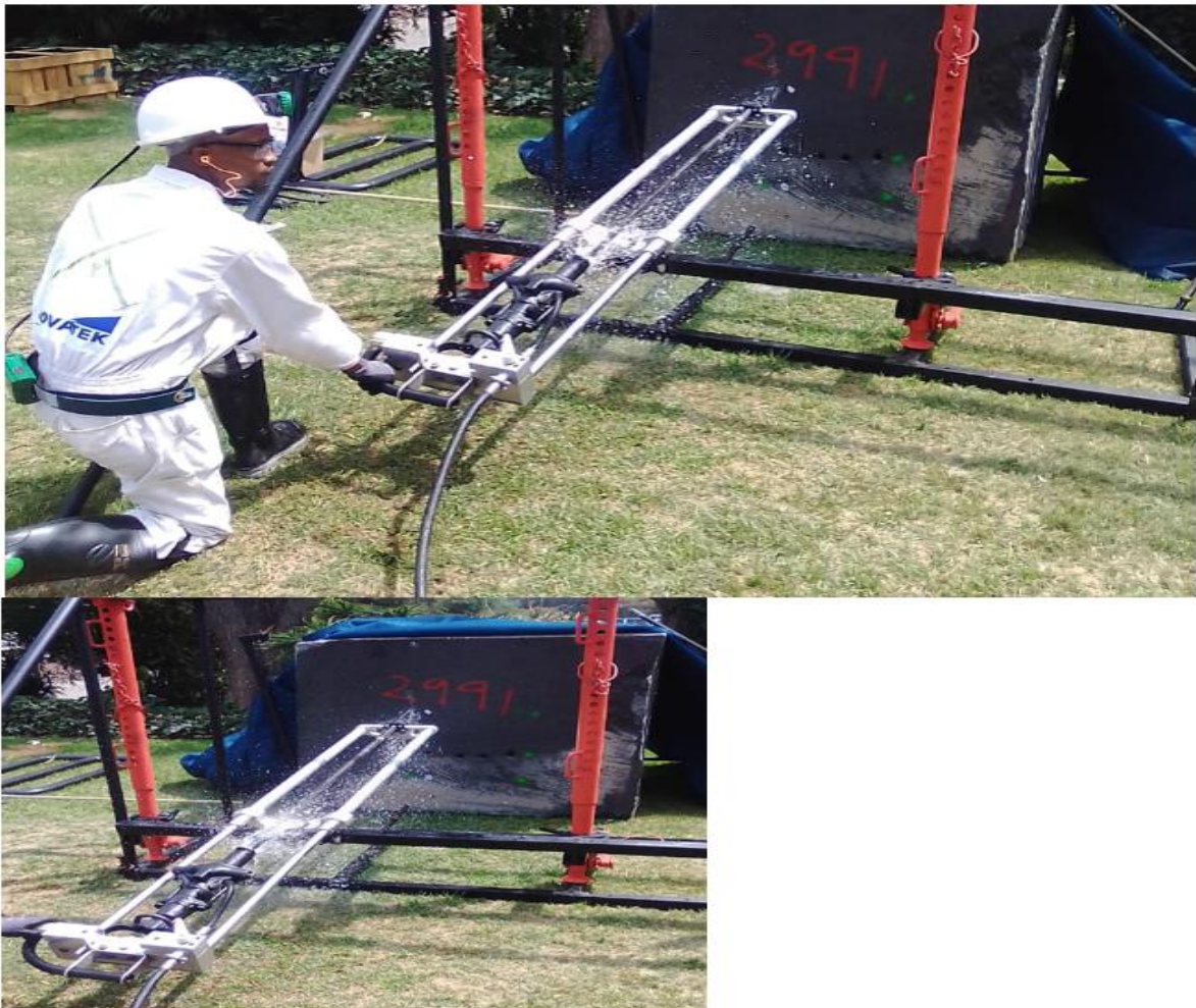
Figure 2: Novatek Isidingo rock drill in operation
