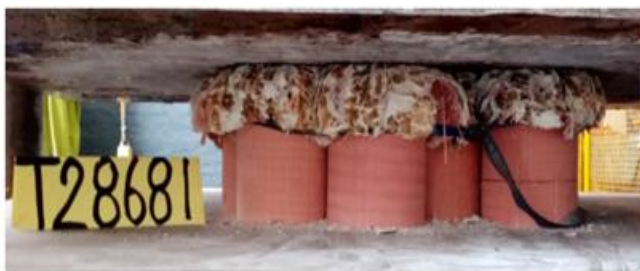
Figure 2. Mine prop composite sticks – fibreglass and resin (400 mm x 170 mm x 10 mm – stack of nine) after the test
