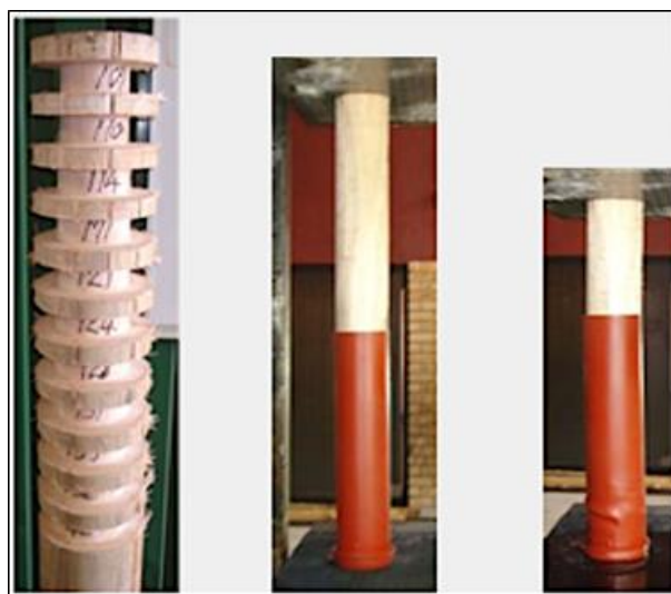
Figure 6. Nimrite timber-based elongate subjected to compressive loading (Timrite, 2019)
