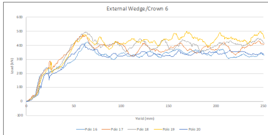
Figure 20: External crown 6 cuts 30mm deep
