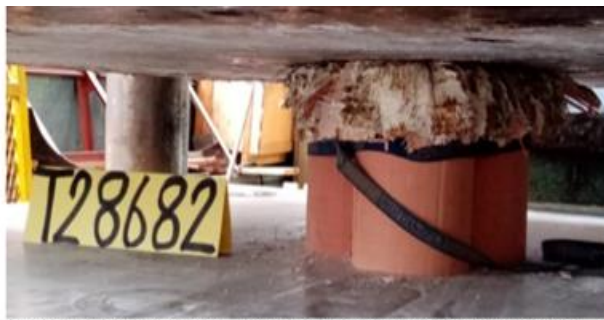
Figure 2. Mine prop composite sticks – fiberglass and resin (400 mm x 160 mm x 10 mm – stack of three) after the test
