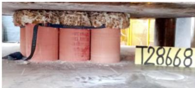
Figure 2. Mine prop composite sticks – fibreglass and resin (400 mm x 170 mm x 10 mm – stack of nine) after the test
