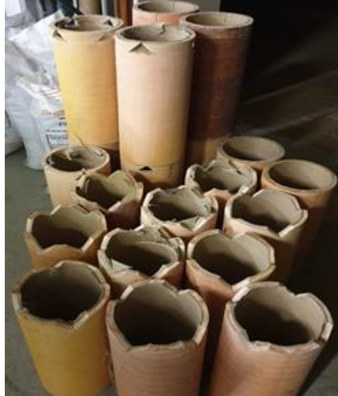
Figure 15 Modified Pole ends. (Cardboard 170mm diameter and laminates were 10mm thick)
