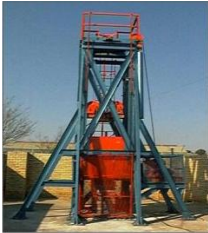
Figure 9: Drop weight (free fall) rig at Timrite.
