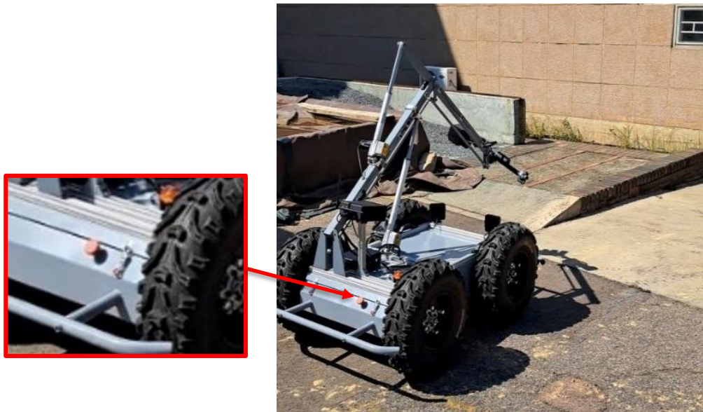
Figure 3. Emergency cut-off switch (Back of RCU) (Els, et al., 2023)
