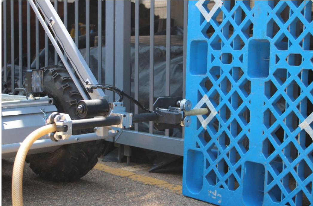
Figure 12. Inserting the charging lance into the identified hole to simulate charging (Els, et al., 2023)
