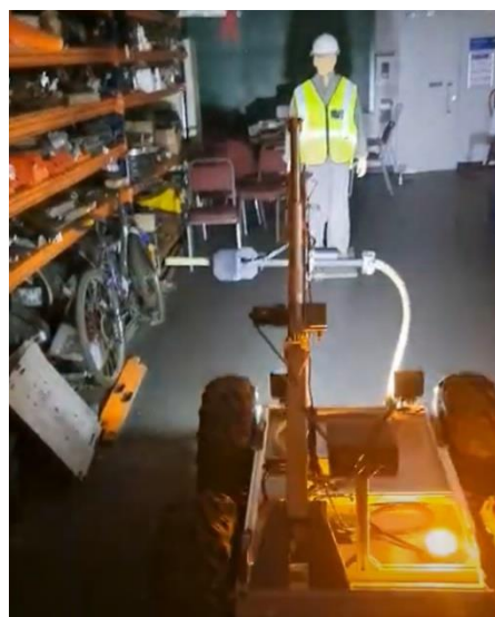
Figure 8. Image of pulsing strobe light on RCU (Els, et al., 2023)
