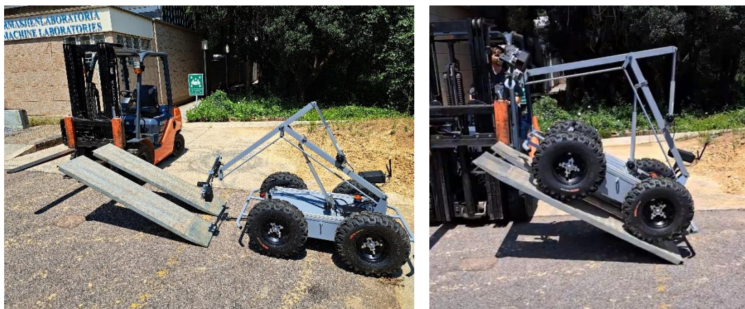
Figure 17. Slope test (drive on steel ramps until maximum inclination is determined) (Els, et al., 2023)
