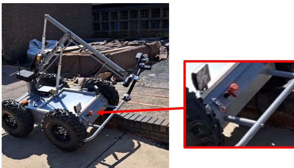
Figure 4. Emergency cut-off switch (Front of RCU) (Els, et al., 2023)
