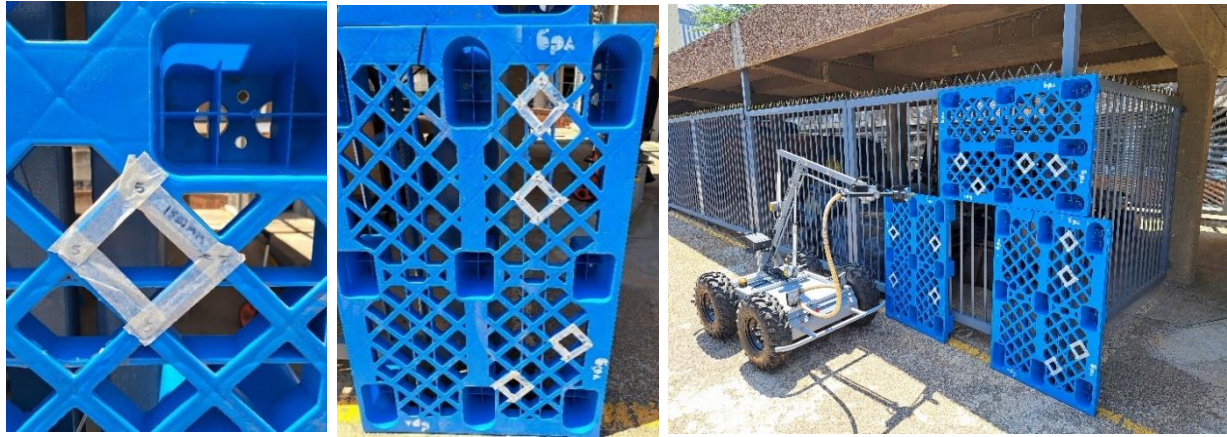
Figure 10. Set-up of artificial stope panel with artificial drilled holes (Els, et al., 2023)
