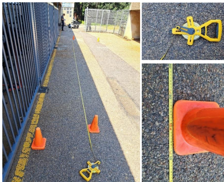
Figure 5. Set-up of a 10 m track to test speed and braking of the (Els, et al., 2023)
