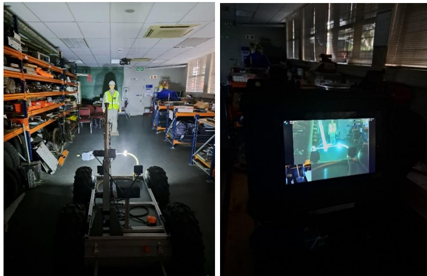
Figure 7. Low light testing of RCU (Left: RCU, right: Operator video feedback) (Els, et al., 2023)
