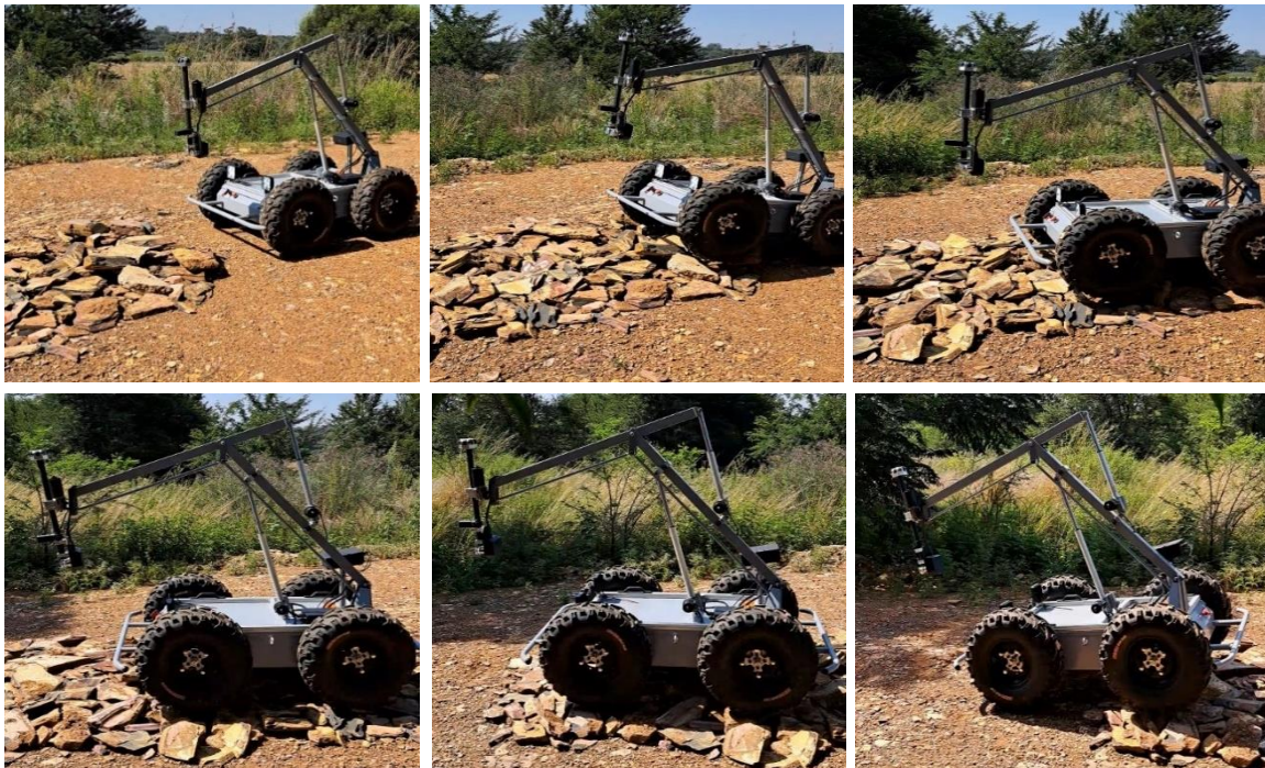
Figure 15. Rough terrain test (driving over a constructed rough, rocky road) (Els, et al., 2023)
