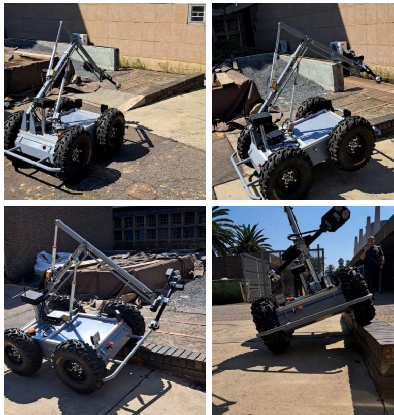
Figure 16. Obstacle and tilt test (driving at an angle with two wheels on an elevated surface and the other two wheels on the ground) (Els, et al., 2023)
