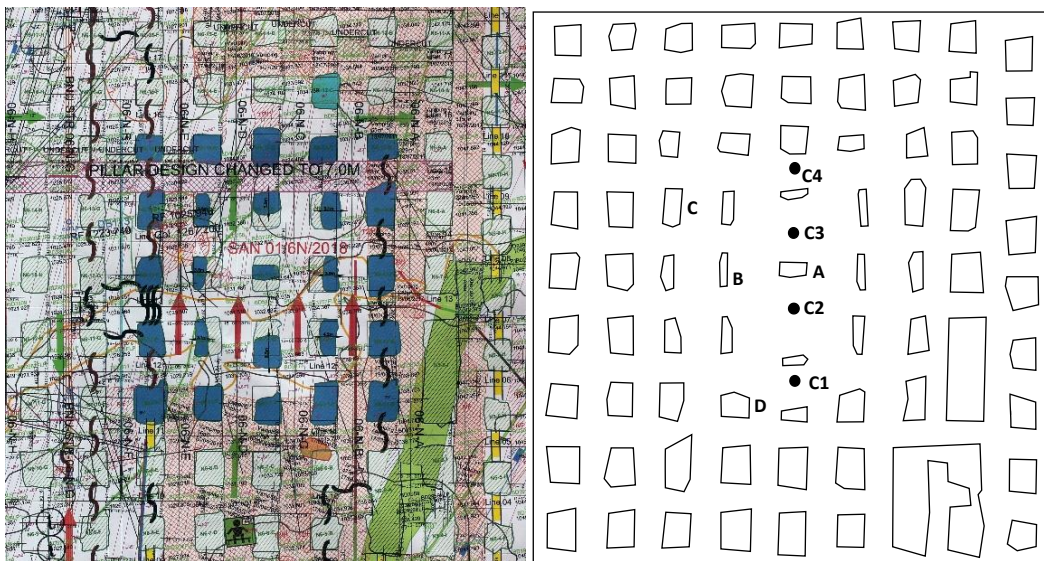
Figure 28. Layout of the experimental pillar mining area where pillars in blue were gradually reduced in size to increase the load on the central pillar. The final geometry of the experimental area when the experiment was terminated is shown on the right (after Napier and Malan, 2021)
