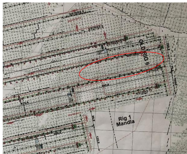
Figure 80. Layout in the experimental area where slipping of the UG2 pillars were done
