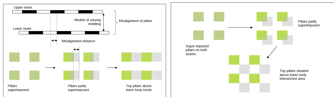
Figure A7. Pillar misalignment considered for pillar interaction on seams
