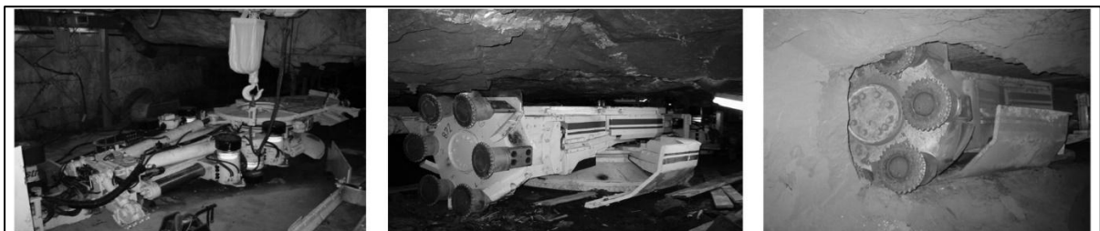
Figure 32. Images depicting the assembly of the ARM1100 and cutting into the rase (Moxham, 2004)
