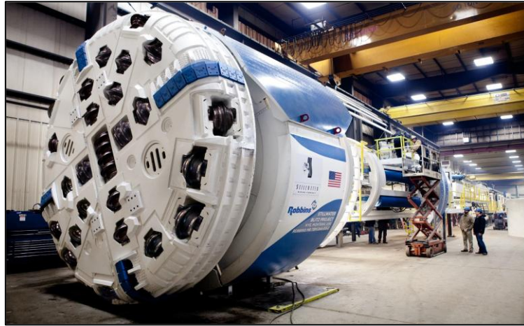
Figure 58. Image showing a TBM for a specific mining application (Robbins, 2024).
