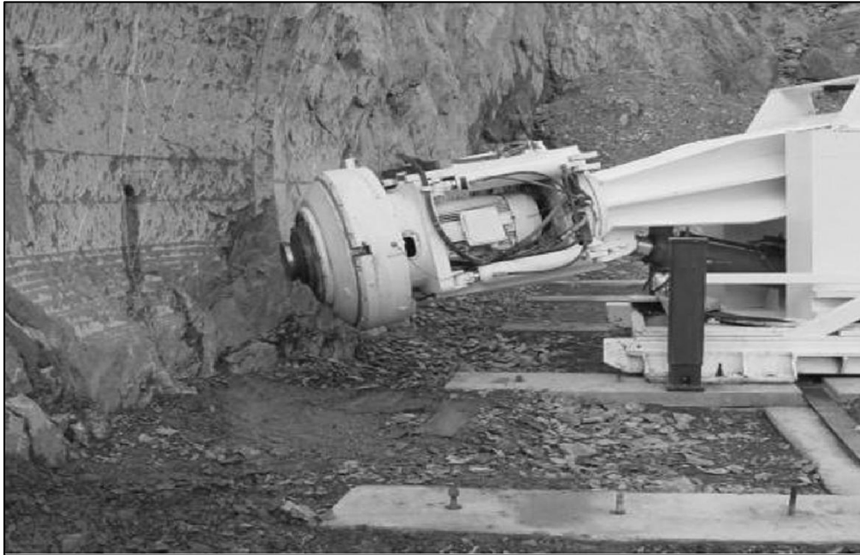
Figure 27. Oscillating disc cutter (Croll, 2004)
