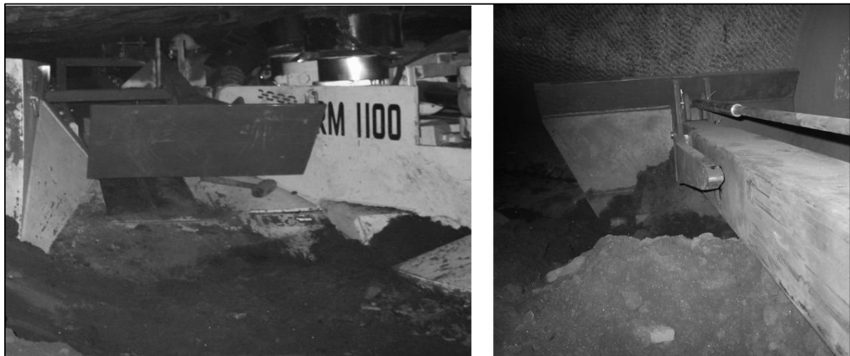
Figure 39. Images of the scoop used to load cuttings onto the conveyor (Moxham, 2004)
