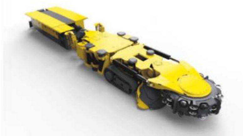
Figure 46. Epiroc Mobile Miner tested at Anglo's Twickenham mine (Lyly et al., 2018)
