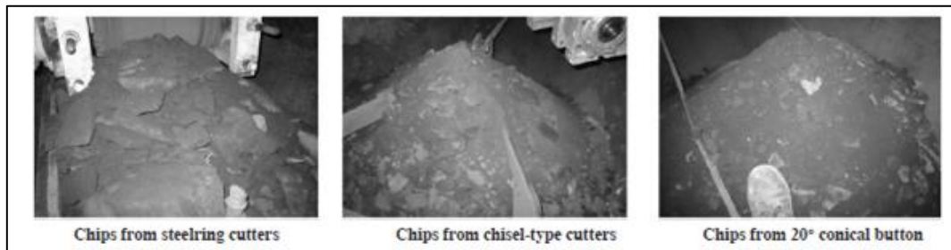
Figure 36. Variations in rock fragments produced due to alternative cutter set-up
