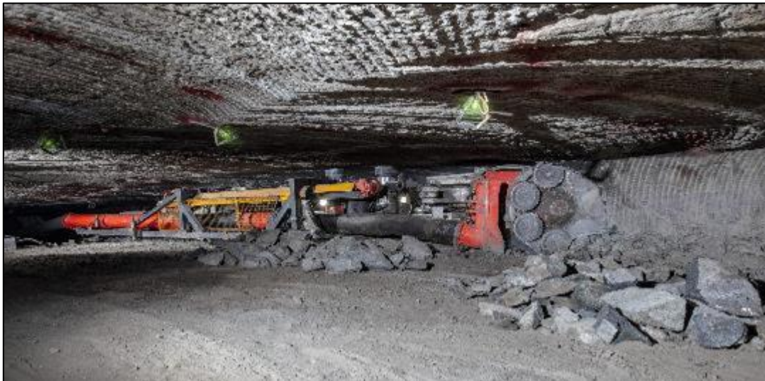
Figure 57. Front view image of the Sandvik MM220 reef miner underground at Twickenham mine (Anglo American, 2024)
