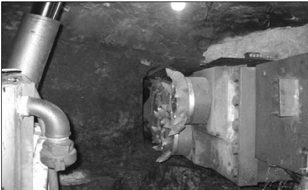
Figure 28. Activated drum system (Croll, 2004)
