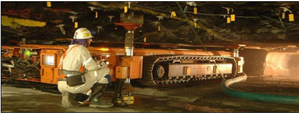
Figure 56. Rear view image of the Sandvik MM220 reef miner underground at Twickenham mine (Anglo American, 2024)
