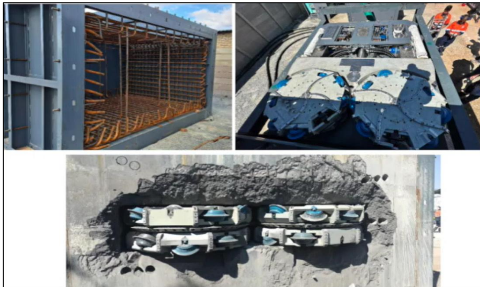
Figure 55. Master Drilling production cutter head testing (Van der Bijl, 2024)
