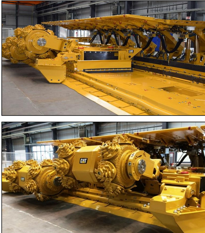
Figure 40. Images of Caterpillar's HRM220 Longwall Hard Rock Mining Machine
