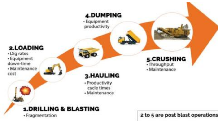
Figure 5: Drilling and Blasting of the mineral extraction process (Bhandari et al., 2017)
