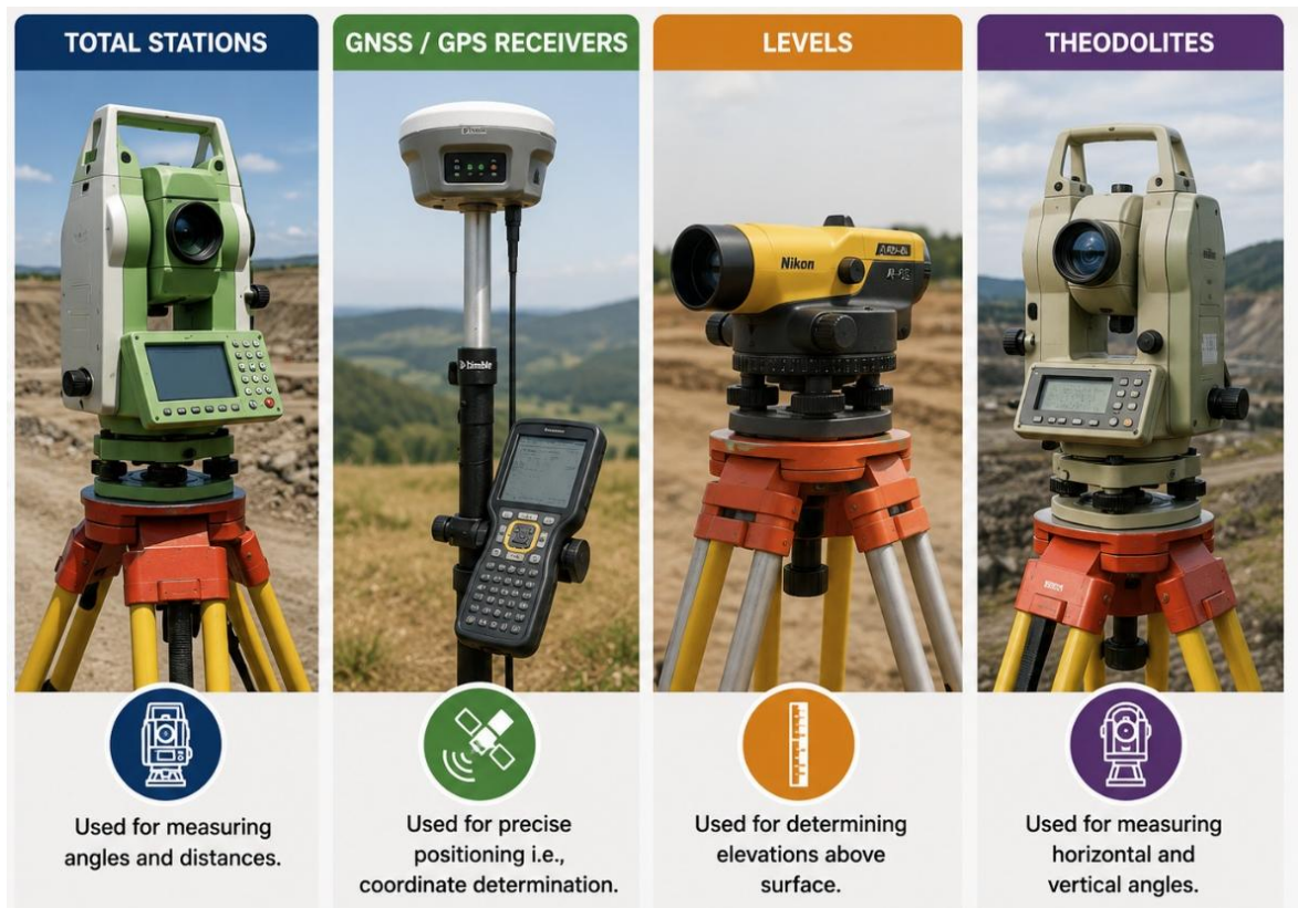
Figure 4. Commonly used survey equipment described at the survey lab.
